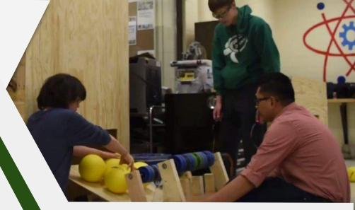
After trying many different prototypes, we settled on a double-axle shooting system. Similar to a baseball shooter, this means that there are wheels on both sides of the shooter to help the ball fly up into the air.
